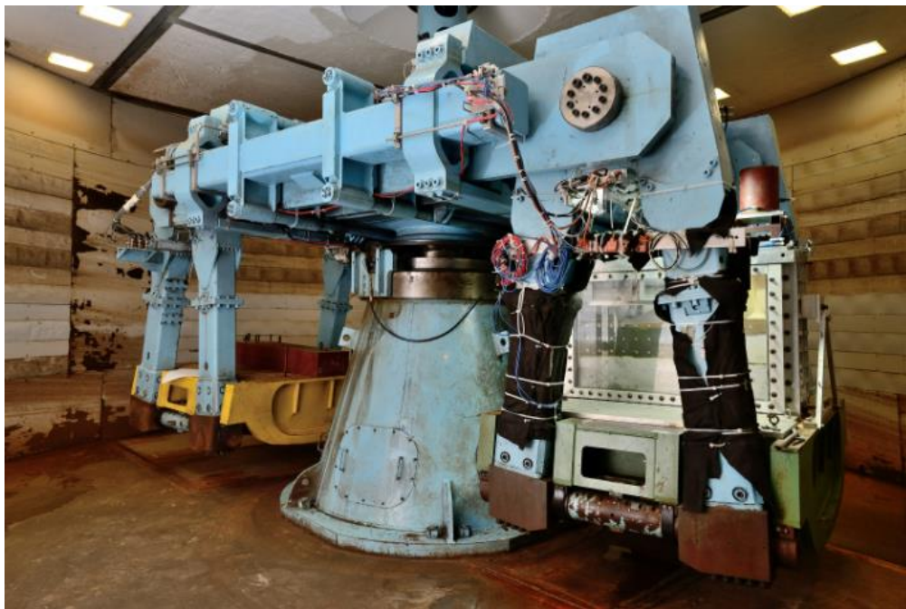
Plate 1. The 8.5 m-diameter (400g-ton) beam centrifuge at the HKUST
